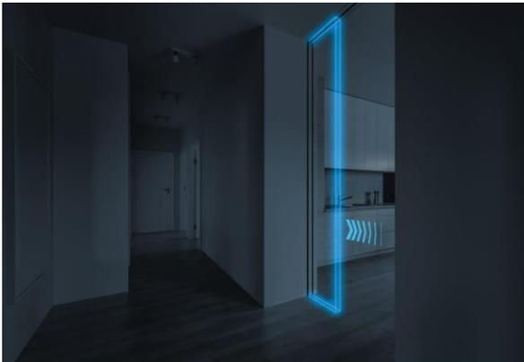
**PushPlus** is another innovative solution from Titus for pocket doors. Typically, a pocket sliding door in a fully open position stops slightly before the wall hollow, protruding and obstructing the area available for moving. PushPlus system allows the door to be without a handle and to retreat entirely into the wall. To close, you activate it with a push. For maximum comfort, safety, and silence in use, the same system also provides damping in the opening direction.
